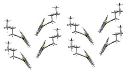
Figure 10. Packing of molecules of B 2 T 3 as seen down the long molecular axis. The stacking direction is vertical in the picture, and the herringbone-like structure occurs in pairs of stacks to give a “lamellar herringbone” structure.
